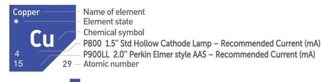
Colour denotes elements that can be made into Hollow Cathode Lamps
